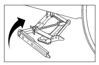
Raise the vehicle by turning the wrench clockwise. Raise the vehicle far enough off the ground so there is enough room for the compact spare tire to fit.
